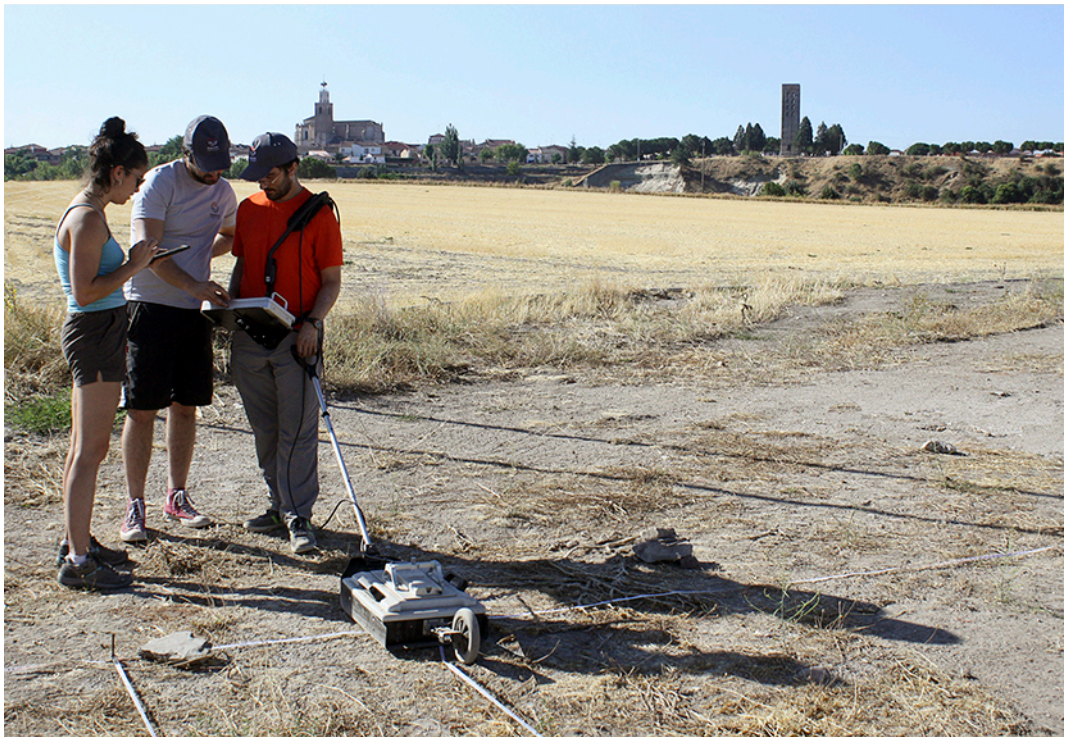
Figure 3. Ground Penetrating Radar Survey at Las Pizarras. Surveyors and a team member during the data collection.
